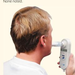
Single use mouthpiece for each person. 6–12-monthly calibration required using CO calibration gas cylinder.
